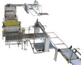
Lines for Panel Lamination (veneers, laminates and papers)
